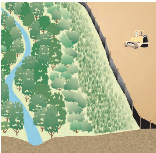
Figure 7. Protect vegetated buffers by using silt fence or other sediment controls.
